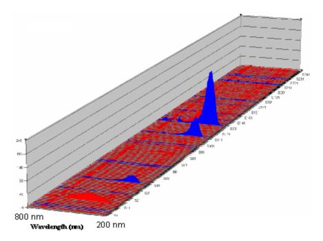
Figure 2: 250 successive single-shot fluorescence spectra from ambient aerosols (NRL on Aug. 18, 2004) illuminated by the 263 nm Q-switched Nd:YLF laser (50  $\mu$ J/pulse). The blue spectra are the detected ambient aerosol particles having bio-threat-like fluorescence spectra, while the red spectra are from non-bio-threat-like particles.
