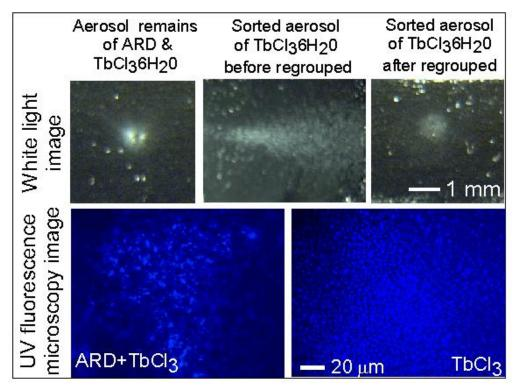
Figure 3: The images and microscopic fluorescence images of the un-deflected & deflected aerosol particles of  $TbCl_3 \cdot 6H_2O$  and Arizona road dust (ARD).
