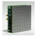
device outputs to the PhotoniQ. Bias to SiPM array is provided by an on-board adjustable high voltage bias supply. A special currentsense output on the supply is available that represents the AC
