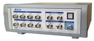
The PhotoniQ Model DAQXY504 is designed to offer scientists, engineers, and developers an off-the-shelf solution for their multi-channel electro-optic sensor needs. Implemented as a stand-alone laboratory instrument with a PC interface, the PhotoniQ is used for charge integration and data acquisition (DAQ) from Anger logic-connected multianode photomultiplier tubes (MAPMT) and silicon photomultiplier (SiPM) arrays. The use of Anger logic allows for high channel count
